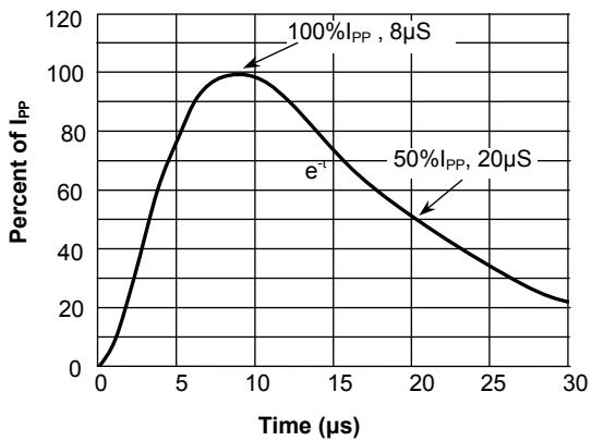
**Fig.4 Pulse Waveform-ESD(IEC61000-4-2)**
