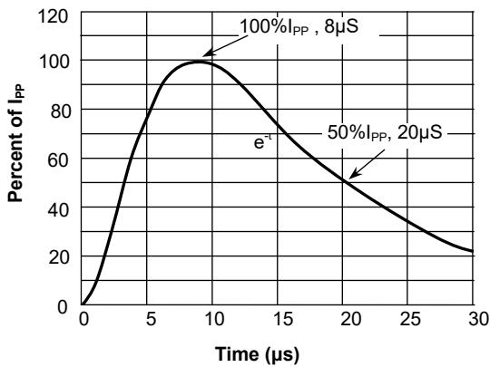
**Fig.4 Pulse Waveform-ESD(IEC61000-4-2)**
