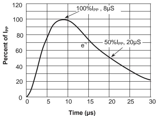
**Fig.4 Pulse Waveform-ESD(IEC61000-4-2)**
